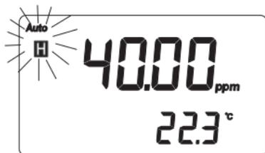
When the reading is stable, the “Auto” and “H” tags stop blinking and the reading is frozen.
