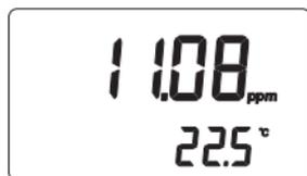
For accurate DO measurements, a water movement of 0.3 m/s is required. This is to ensure that the oxygen-depleted membrane surface is constantly replenished. A moving stream will provide adequate circulation.
