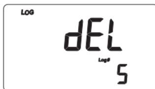
**Note:** Pressing SHIFT and SETUP keys, the instrument toggles between record number and “del ALL”.
