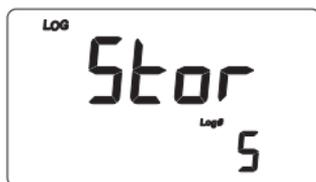
A complete set of information is memorized: date, time, DO and temperature readings.
